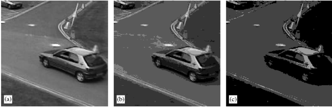
Fig. 1. (a) Input image; (b) image segmented into eight gray level bands; (c) image segmented into four gray level bands.
